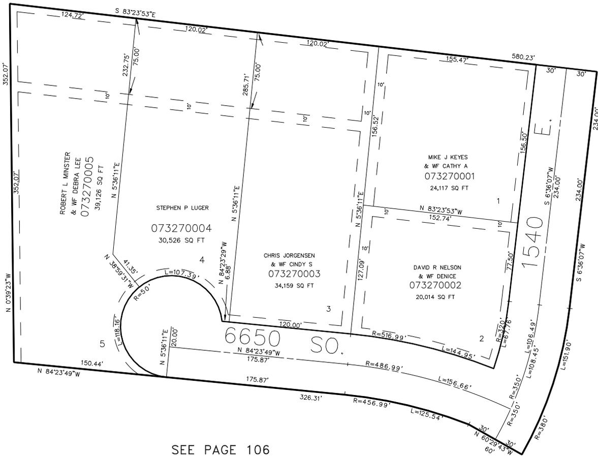
7' UTILITY & DRAINAGE EASEMENTS EACH SIDE OF PROPERTY LINE AS INDICATED BY DASHED LINES OR AS OTHERWISE SHOWN.
